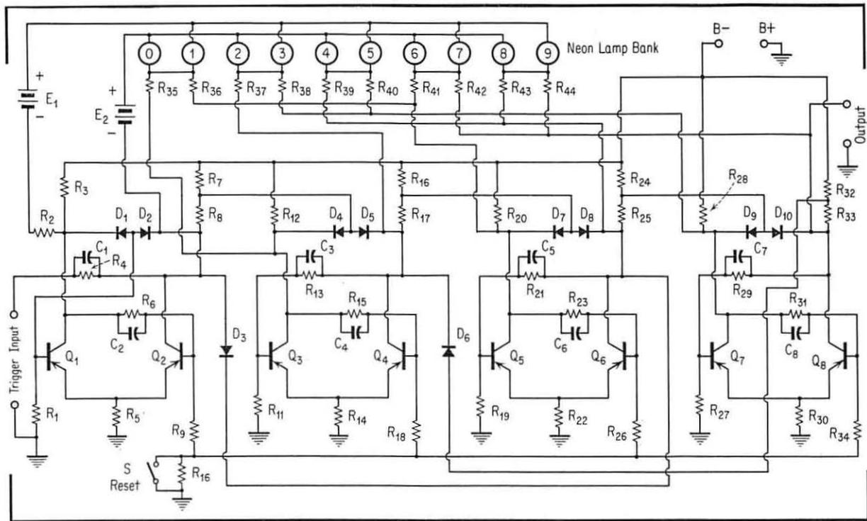
Fig. 4. Transistorized Decimal Scaler.
