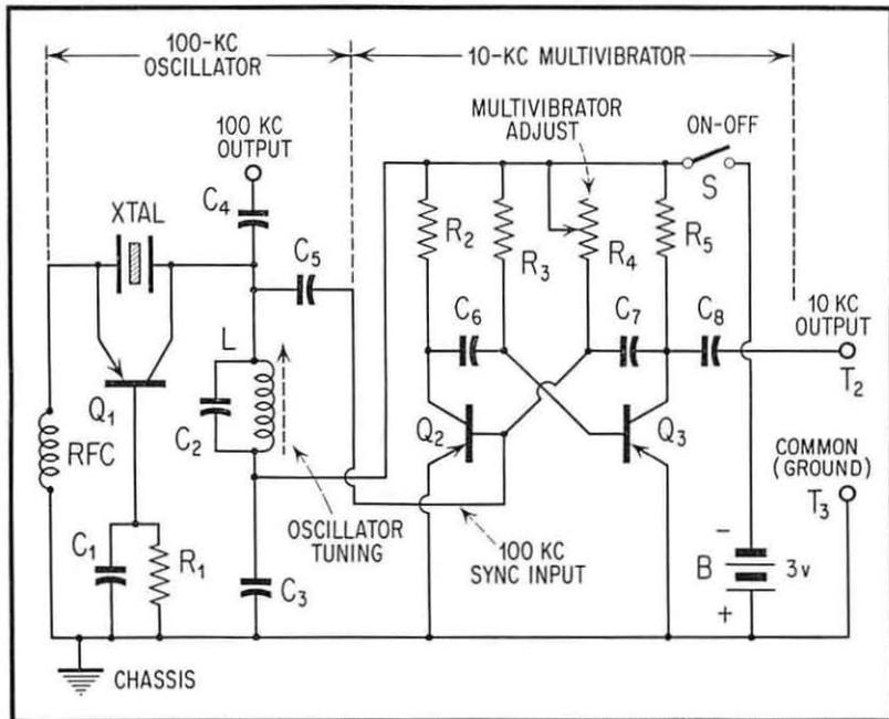
Fig. 3. Complete Circuit of the Frequency Standard.
