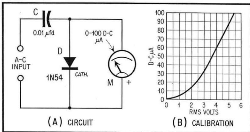
Fig. 4. Shunt Diode-Microammeter Circuit.
