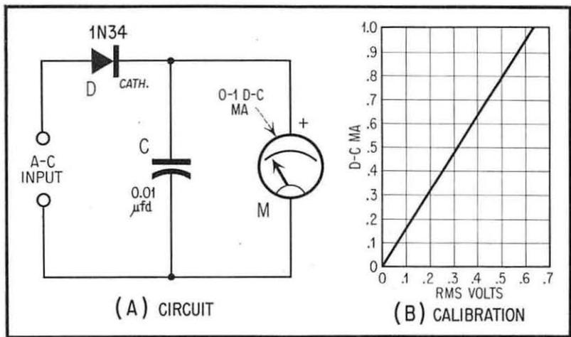
Fig. 1. Basic Single-Diode Circuit with Millimeter.
