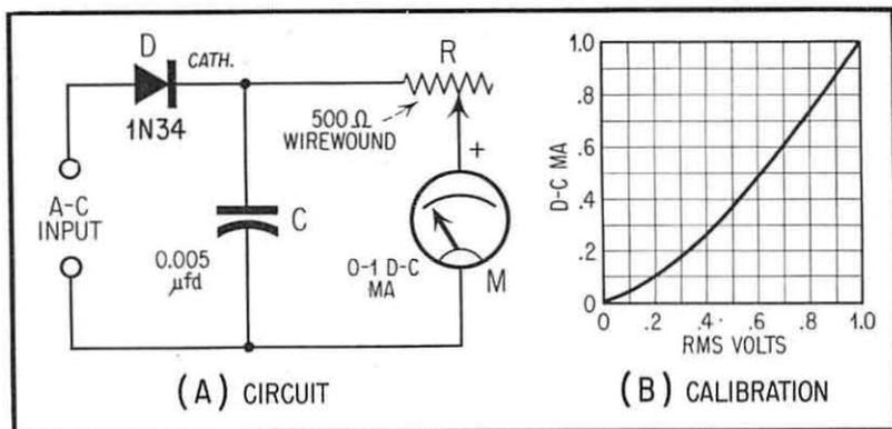
Fig. 2. Diode-Milliammeter Circuit with Multiplier.
