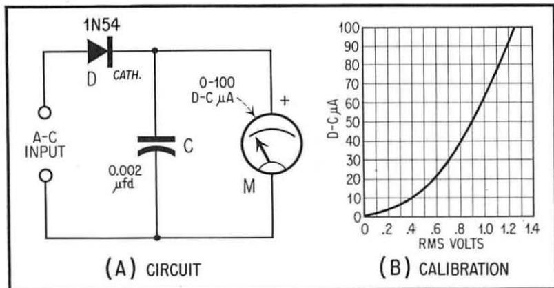
Fig. 3. Series Diode-Microammeter Circuit.
