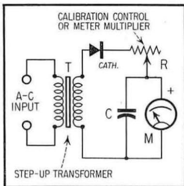
Fig. 9. Transformer-Coupled Diode Millivoltmeter.
