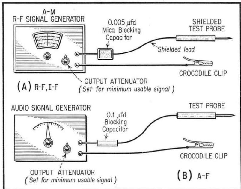
Fig. 2. Signal-Injection Instruments.
