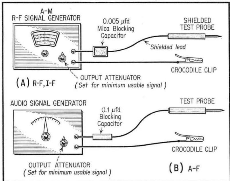
Fig. 2. Signal-Injection Instruments.
