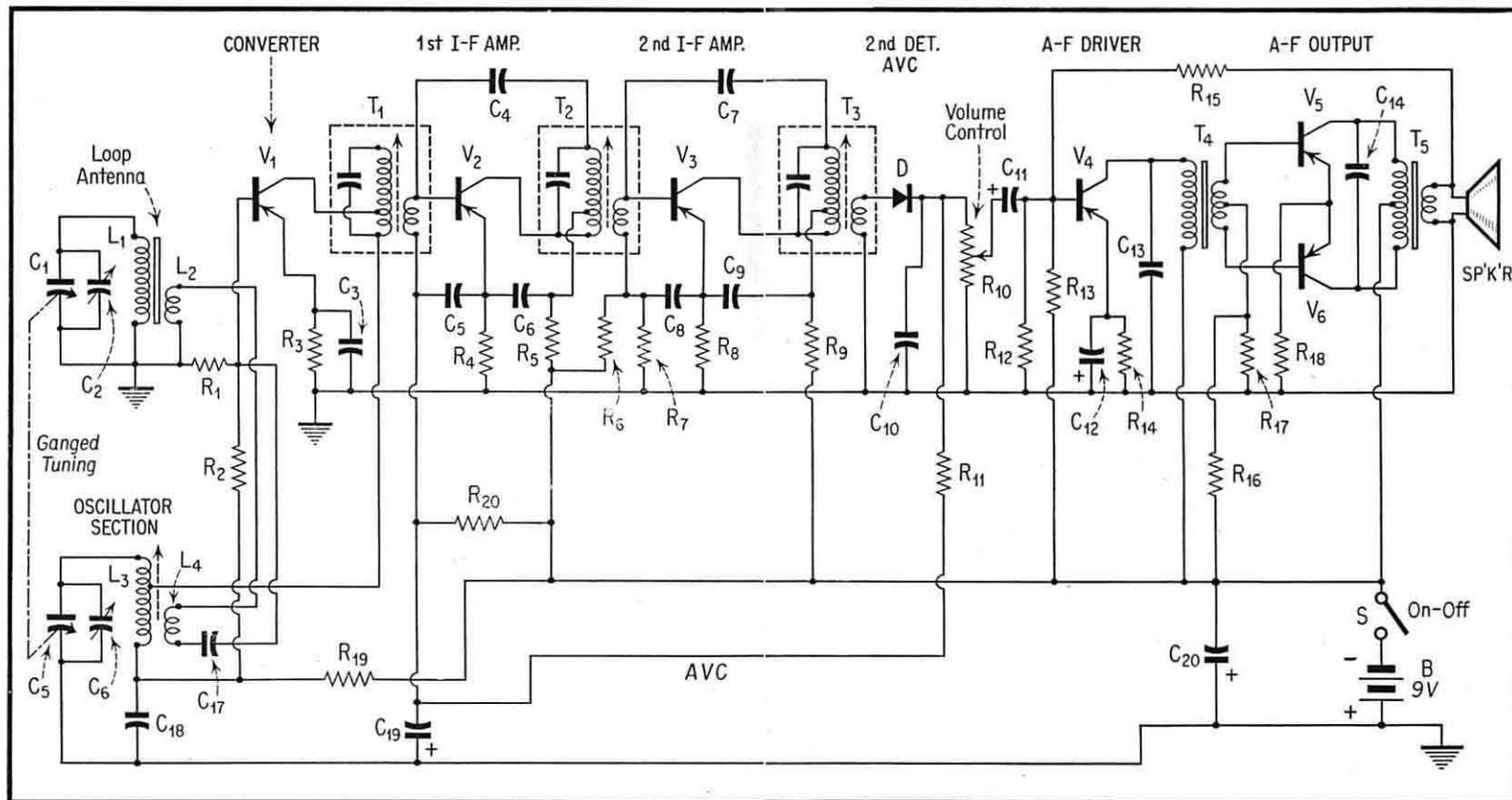
Fig. 1. Typical Transistorized Superheterodyne Receiver.
