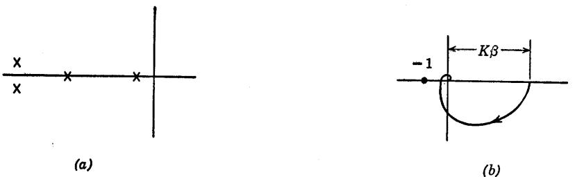
Fig. 12.12. Use of two poles for bandwidth degradation.
