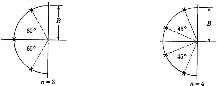
Fig. 5.3. Poles of the maximally flat transfer function.
