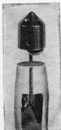
Fig. 78.—Filled Electrode for Lamps Operated with Very High Pressures (Osram, Berlin).
