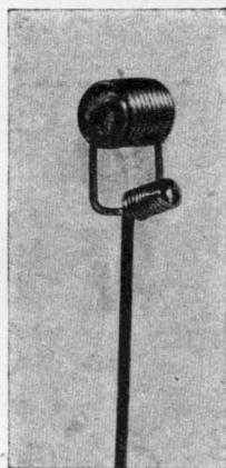
Fig. 74.—Storage Electrode for High-pressure Lamps (Osram, Berlin).
