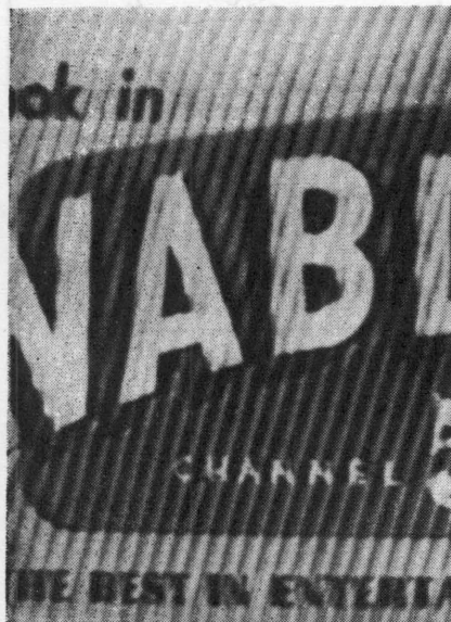
FIG. 1—Interference from third video i-f harmonic on channel 5
