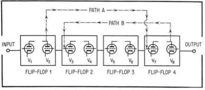
Fig. 2. Arrangement of Decimal Scaler.
