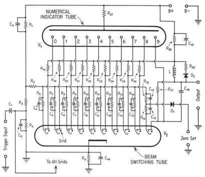
Fig. 6. Beam-Switching Counter Decade.
