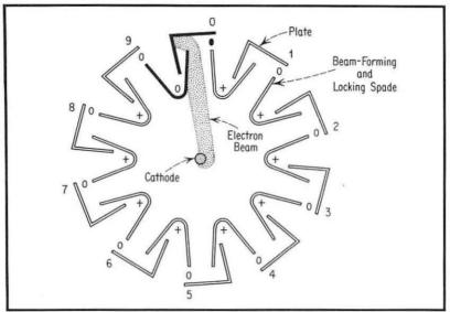
Fig. 5. Details of Beam Switching Tube.
