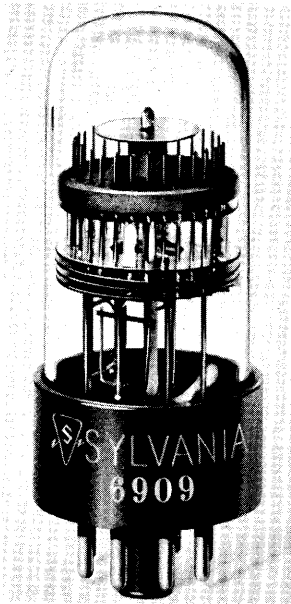
Fig. 136. Multiple-cathode counting glow tube. (Courtesy of General Telephone and Electronic Labs., Inc.)
