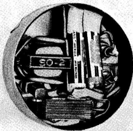
Fig. 603. Inside view showing how the miniaturized components are mounted.
