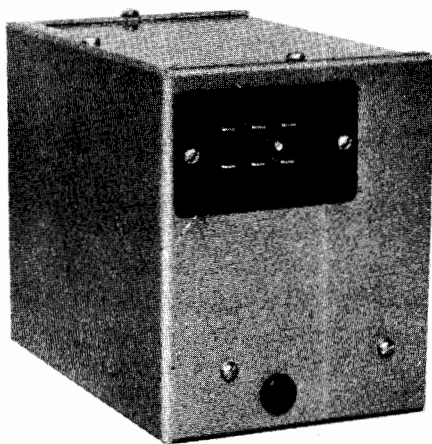
Fig. 702. Exterior view of the control box showing the mounting of the Jones plug. The numbering of the male plug terminals is as follows: across the top, from left to right, 2, 4, and 6. Across the bottom, from left to right, 1, 3, and 5. Note the polarizing pin. This prevents incorrect insertion of the plug.
